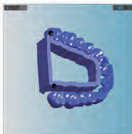
✗ Side support plate height is too high
